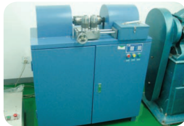
Wire twisting tester for wire twist testing
