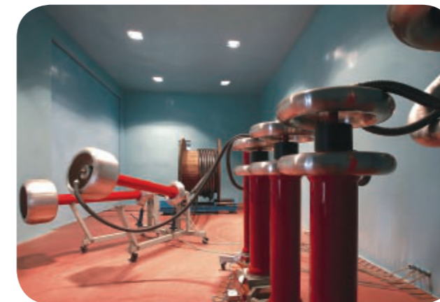
Partial discharge detector for voltage test and partial discharge testing
