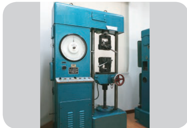
Tensile testing machine for elongation and breaking load
