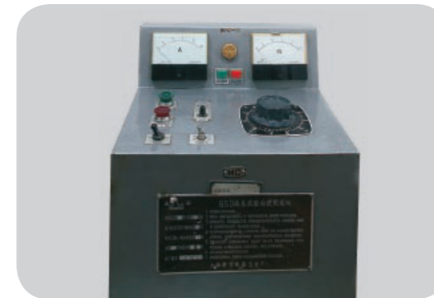
High voltage testing platform
