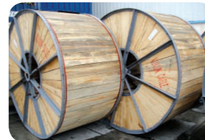
Iron-wooden drum with wooden board lagging
