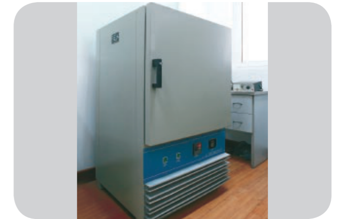
Heat aging oven for before aging and after aging mechanical property
