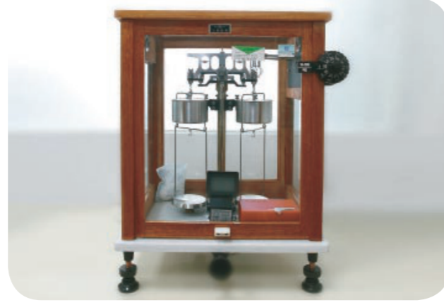
Light-electrical analytical balance for weight and density testing
