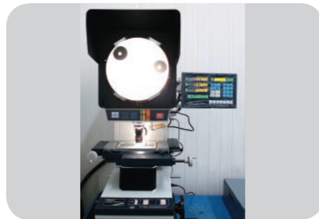
Digital measuring projector for insulation and sheath thickness testing
